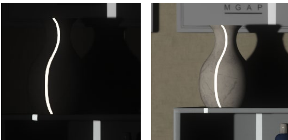
Fig. 32: The background illumination provides a better overview while the slit light is still visible
